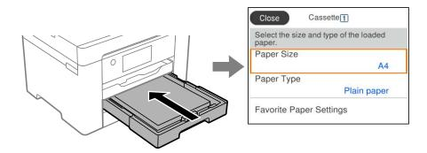
If displayed paper size and type differ from the loaded paper, select the item to change. If the settings match the loaded paper, close the screen.
