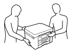
☐ When carrying the printer, do not tilt it more than 10 degrees; otherwise the printer may fall.
